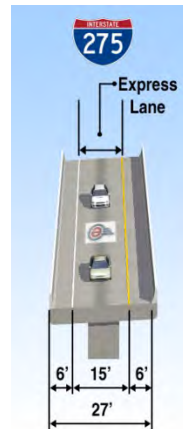
FIGURE 6-14: I-275 EXPRESS LANES TYPICAL SECTION FROM NORTH OF I-4 TO NORTH OF BEARSS AVENUE FPID 431821-2
